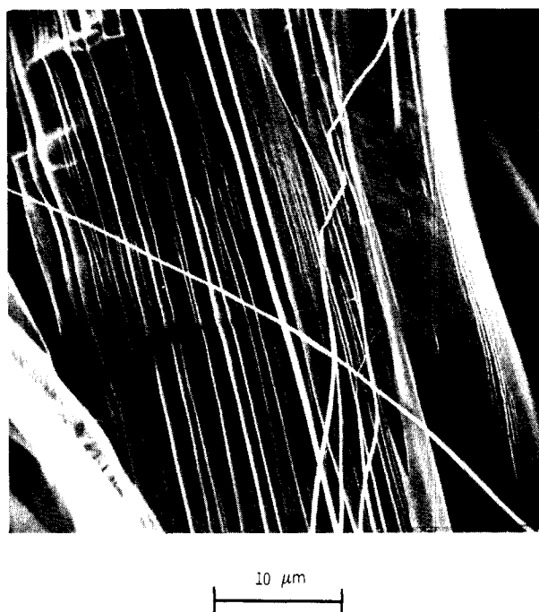
Figure 2. Fractured PBT film. Film was prepared from a 5% PBT/PPA solution by pulling through rollers and then precipitating the solution by dipping in water.
